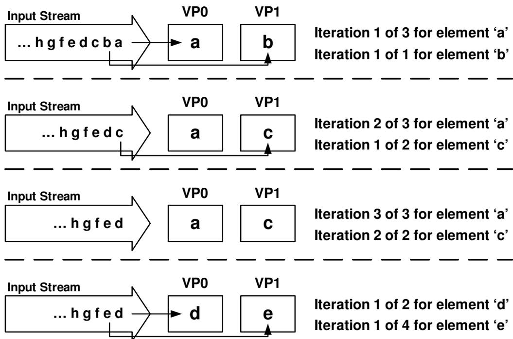
Figure 3.16: Two virtual processors executing the same while-loop, but on different stream elements. This scenario is implemented on a single cluster using loop-flattening and state-unrolling, where the latter duplicates the loop code *and* loop state for each virtual processor.
