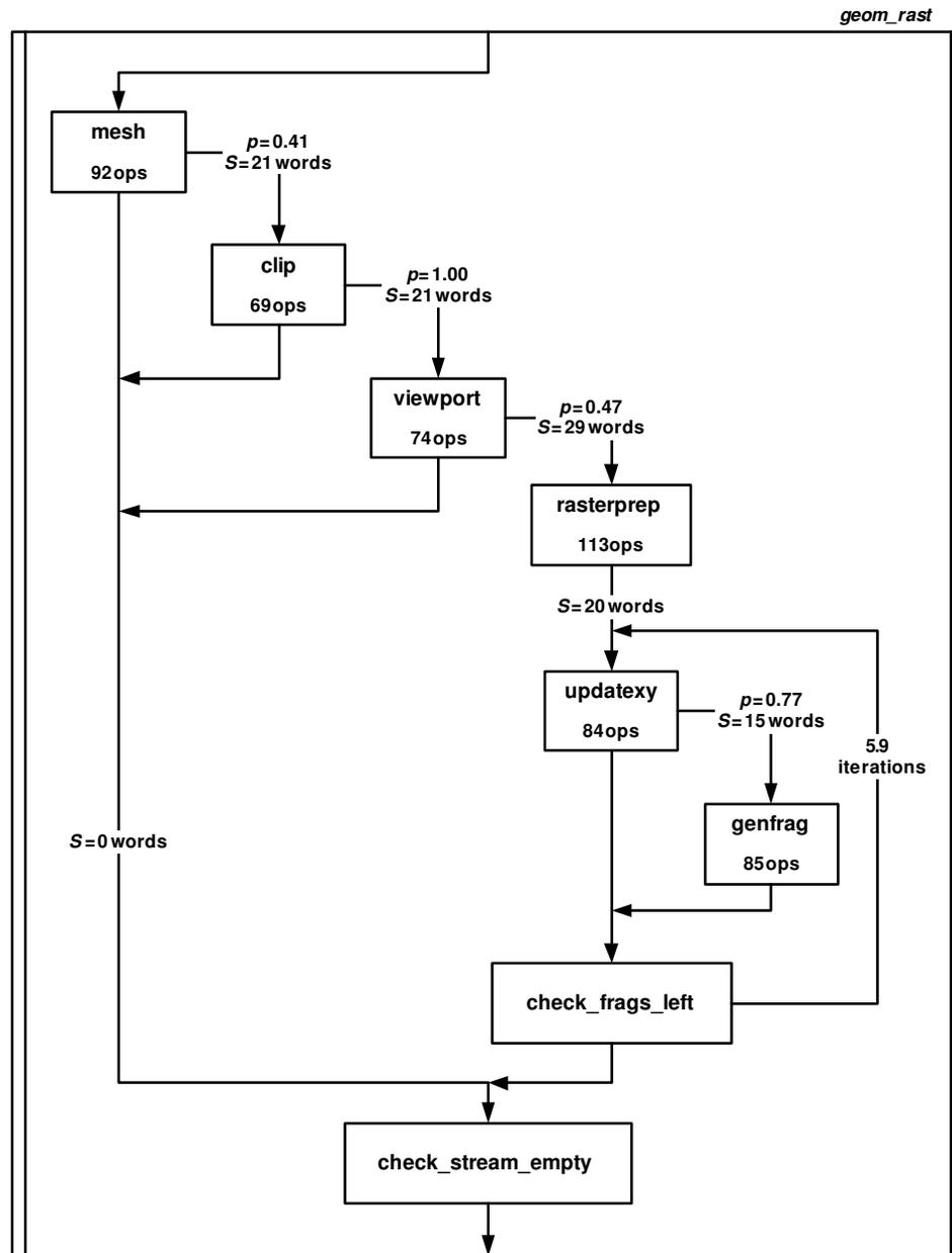
Figure 3.23: Basic block diagram for the *geom\_rast* kernel. The basic block names correspond to those used in Kernel 2.1. Indicated on the diagram are the number of arithmetic operations in each basic block, the amount of live state that is transferred along each control flow path, as well as the probability that each control flow path is taken.
