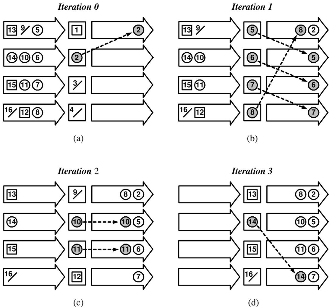
Figure 5.2: This series of figures shows how using a conditional output stream can eliminate load-imbalance for the same example as in Figure 5.1. (a)-(d) shows all four iterations of *compute\_I*, after which the data are balanced between the four SRF banks.
