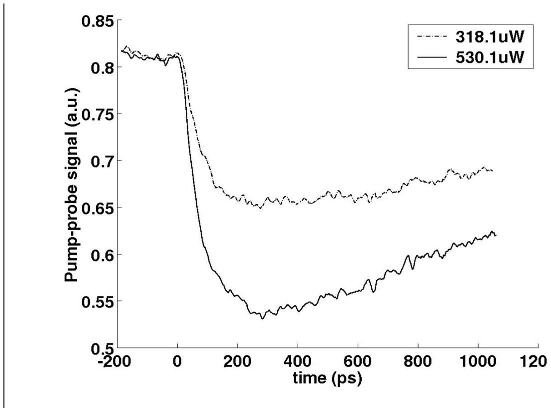
Figure 4.7 Pump-probe measurements of falling edge at the clock input to PRBS clocked by MQW detectors. Powers are per detector; 318  $\mu$ W and 530  $\mu$ W are shown
