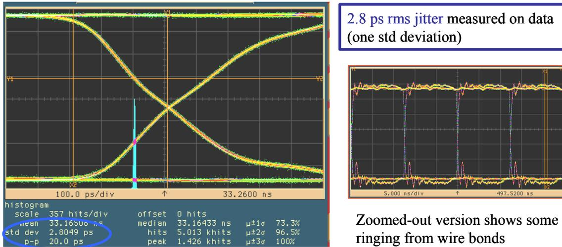
Figure 4.5 Zoomed-in picture of eye diagram of the output of the PRBS driven by the optical clock. The histogram of the jitter on the falling edge is shown. A zoomed out version is also shown
