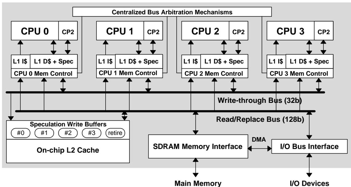
**Figure 2-2: Hydra chip multiprocessor**
