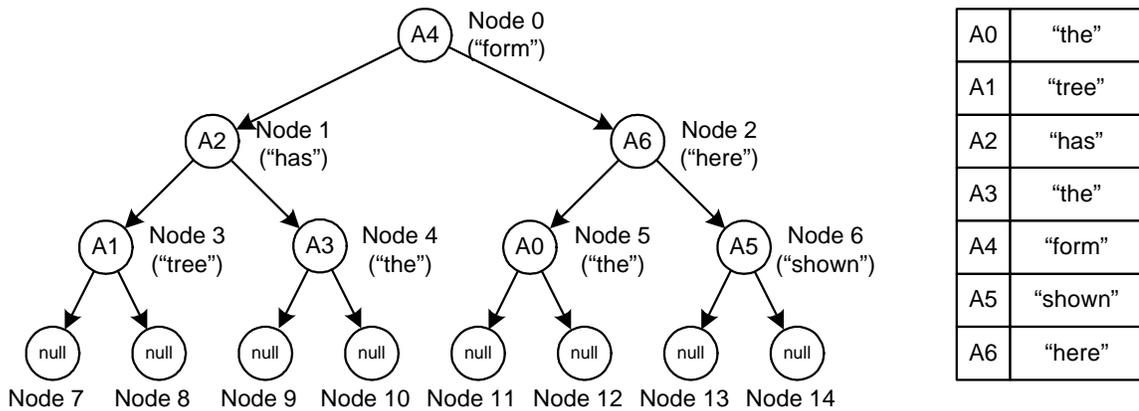
Figure 3-1: Organization of the heap array
