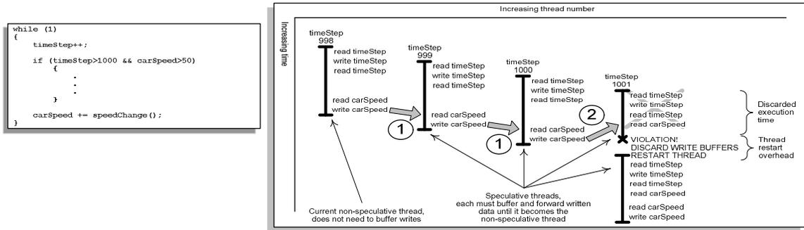
**Figure 2-1: Thread-level speculation**
