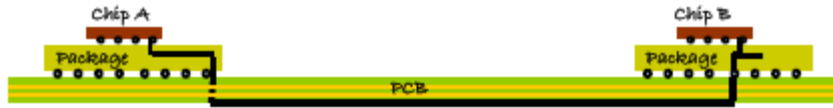
Figure 4.1: A chip to chip system with a dominant stub on the package of chip B.
