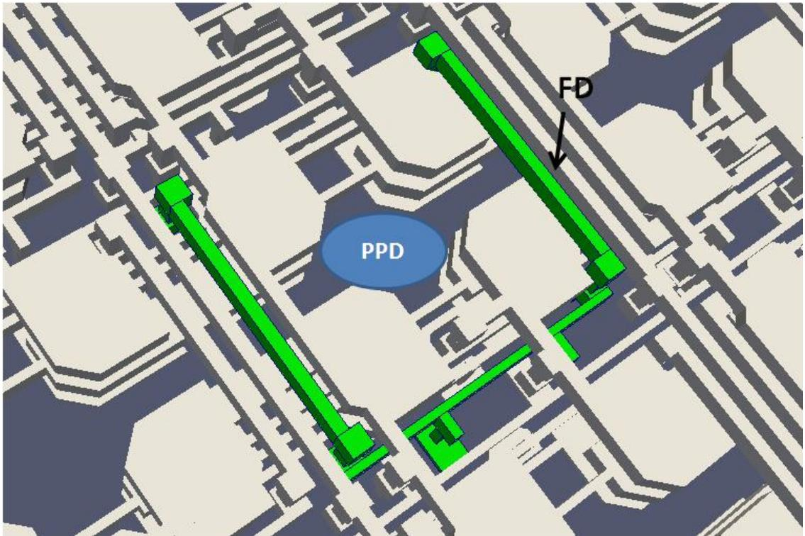
**Figure 4.7:** *Three-dimensional view of the quad-bucket pixel layout. The green line represents the metal used to connect the four floating diffusions of the pixel. For clarity, some signal lines are omitted in this figure.*
