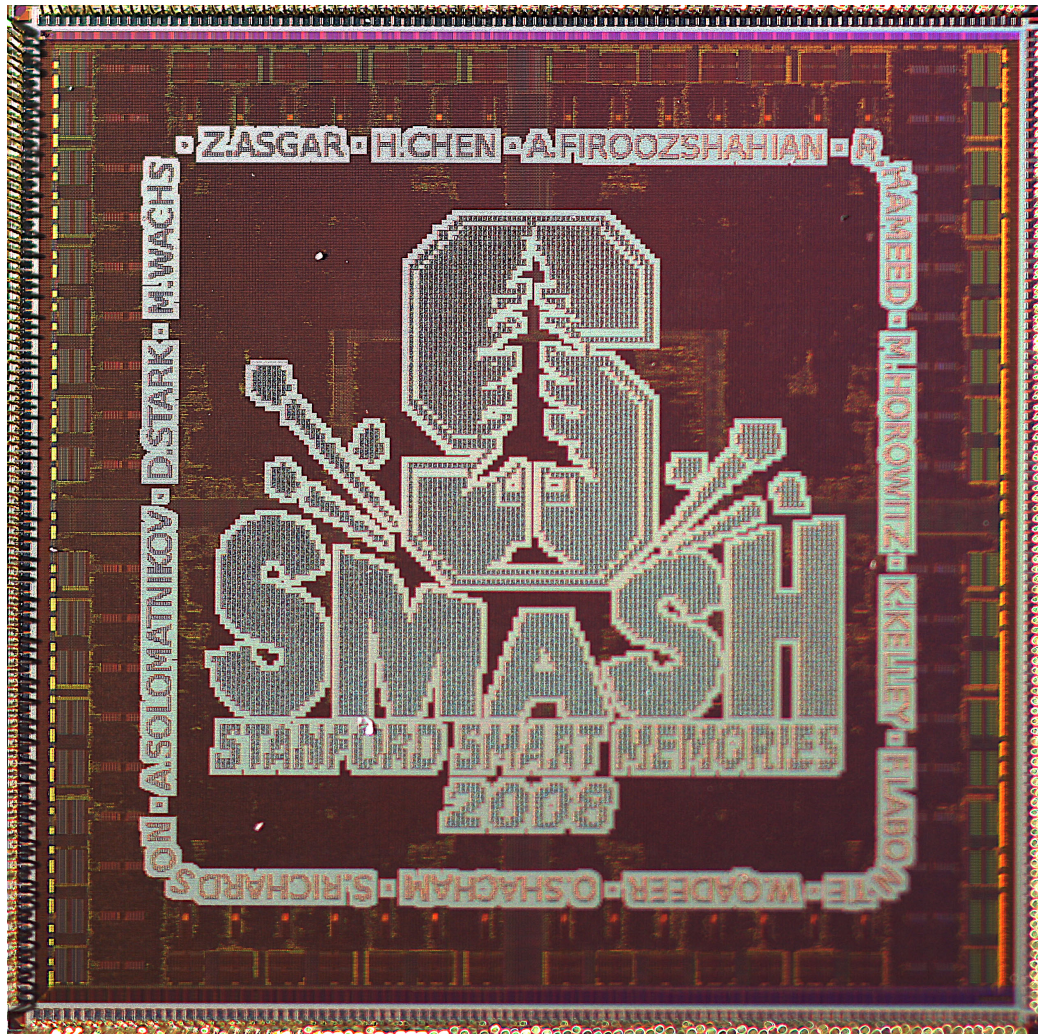
Figure 2.9: Smart Memories Die Photo. The chip was packaged and put into a 4-quad system with 32 processors.
