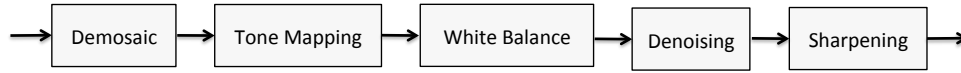
Figure 2.5: Simplified image capture pipeline which converts RAW data from sensor into RGB images or video frames. (TODO: update with a better pipeline)
