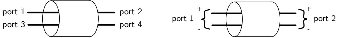
(a) 4-port representation of a lossy channel, where each port represents one side of a data pair. The order shown here is the one typically used in Touchstone files.
