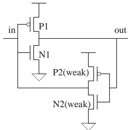
**Figure 3-3.** A Pattern to Find Static Latches and Remove the Weak Feedback
