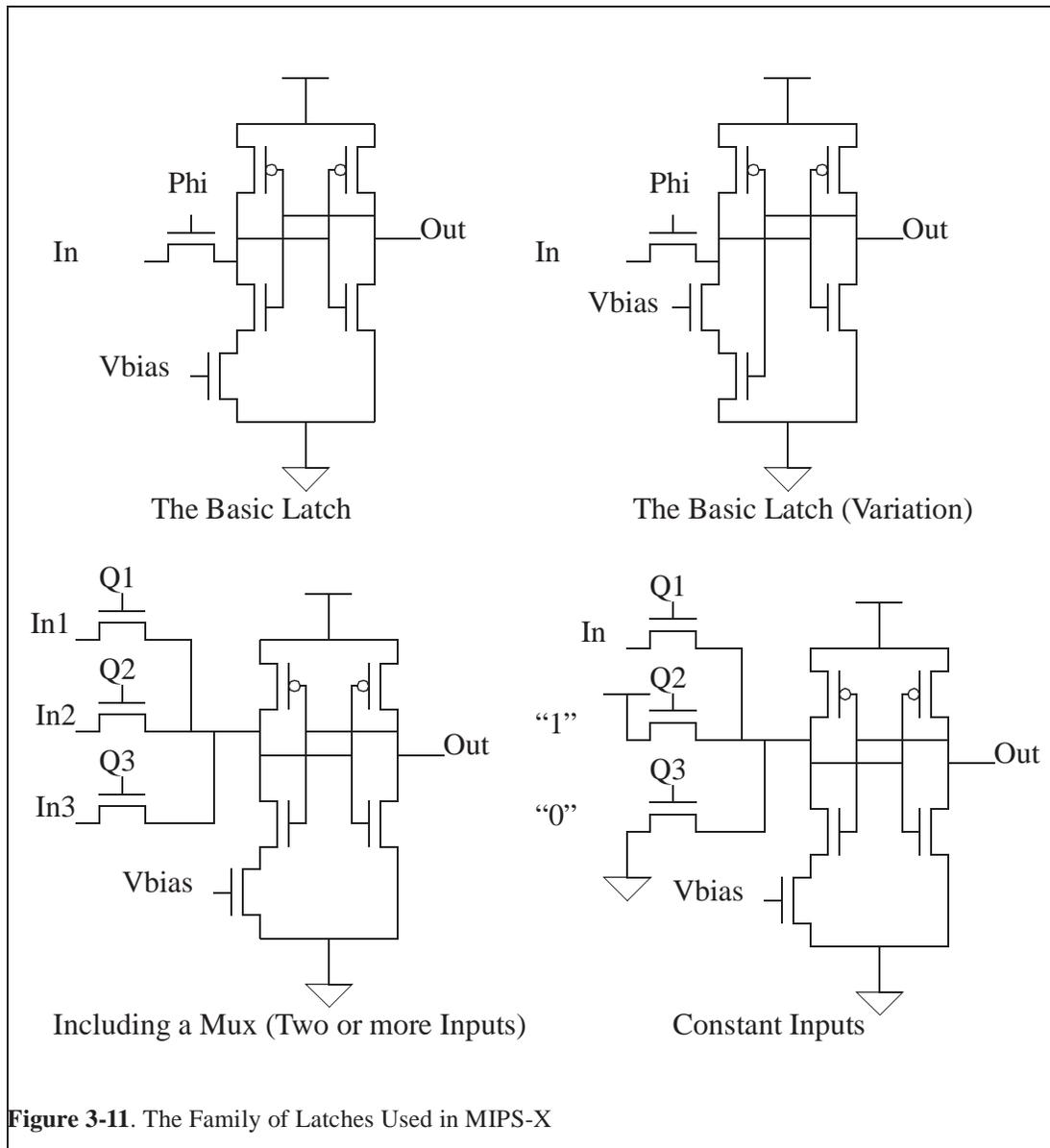
**Figure 3-11.** The Family of Latches Used in MIPS-X
